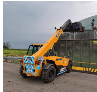
2021: E-Telelader JCB 525, 34 kWh
