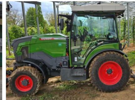
2019..2025: Fendt 100 e 90 PS, 100 kWh
